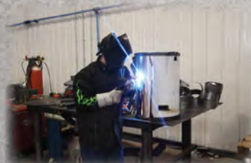
Welding Stainless Steel Housing
