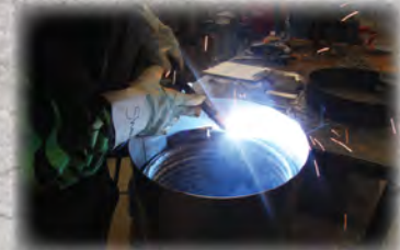
Welding Interior Pipe to Housing
