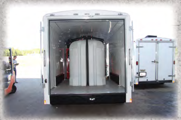
740 Gallon Water Tank
